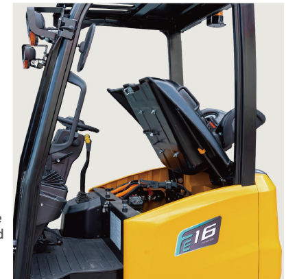
Fully opening electrical control cover for easy maintenance of electric controls and fuses.
