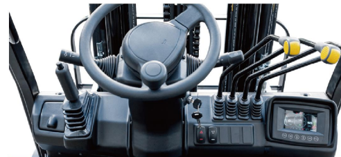
Fully enclosed instrument console greatly expand legroom.
