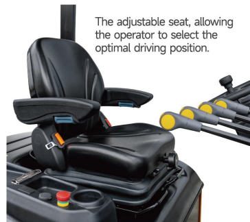
Optional finger-tip control system ensures a superior driving experience.
