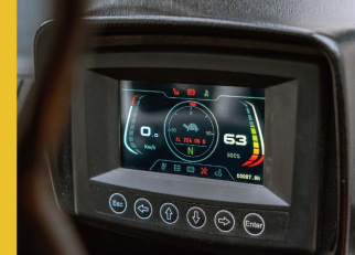
Multi-function color screen instrument provides key information of forklift.
