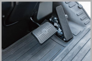
Hanging foot brake achieve smooth braking and reduce vibrations.
