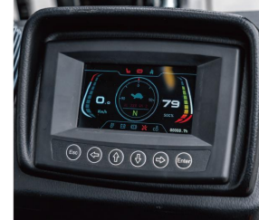
Multi-function color screen instrument provides key information of forklift.
